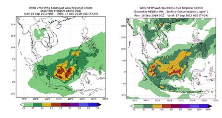
Figure 5 – Example Southeast Asia VFSP-WAC multi-model ensemble median 1-day forecast of smoke AOD (left) and PM<sub>2.5</sub> surface concentration (right) for the Southeast Asia region in September 2019.
